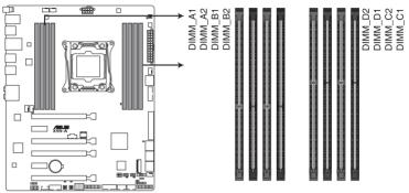
X99-A 288-pin DDR4 DIMM socket
